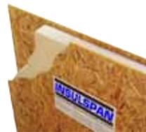
With a solid core of expanded polystyrene insulation and minimal framing, the Insulspan SIP System greatly reduced both thermal bridging and air leakage. To meet the Passive House certification, homes must have air infiltration less than 0.6 ACH50, as confirmed by a blower door test.
