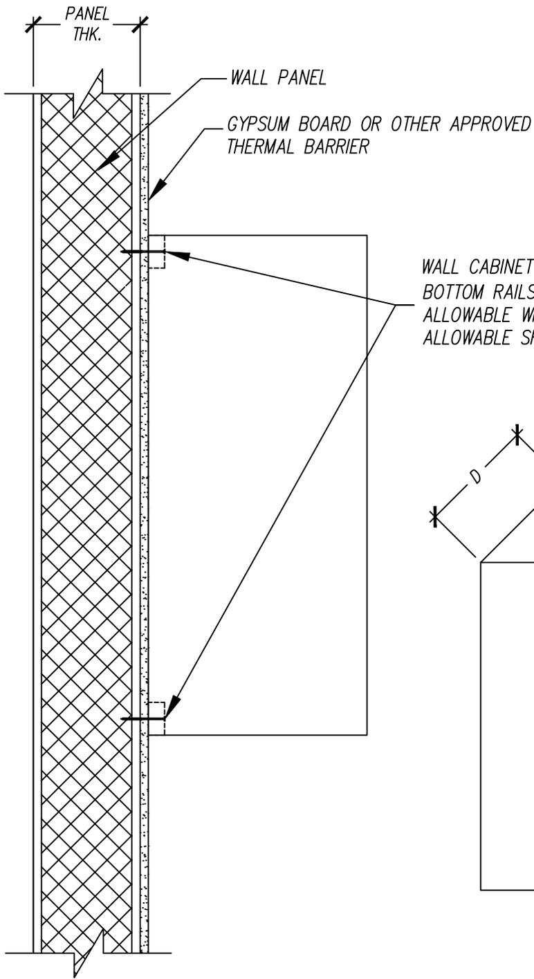
WALL CABINET INSTALLED WITH #8 x 2" DECK SCREWS TOP & BOTTOM RAILS (1x2) SPACE AS REQUIRED
